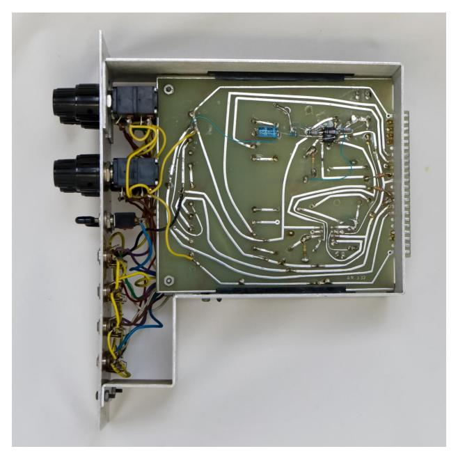
The additional circuitry on the PCB rear is a gain & level shift circuit for VCO B as the potted module is not functioning to specifications
