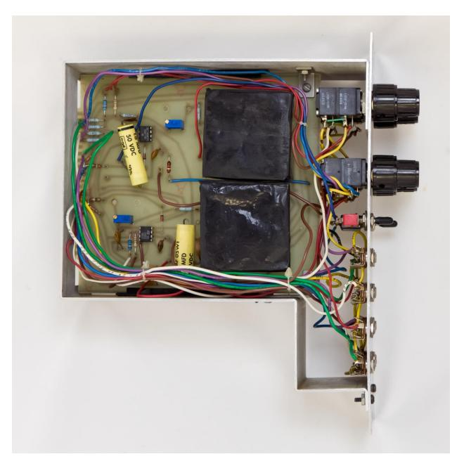
BOth 1 turn trimmers have been replaced with 20 turn trimmers
